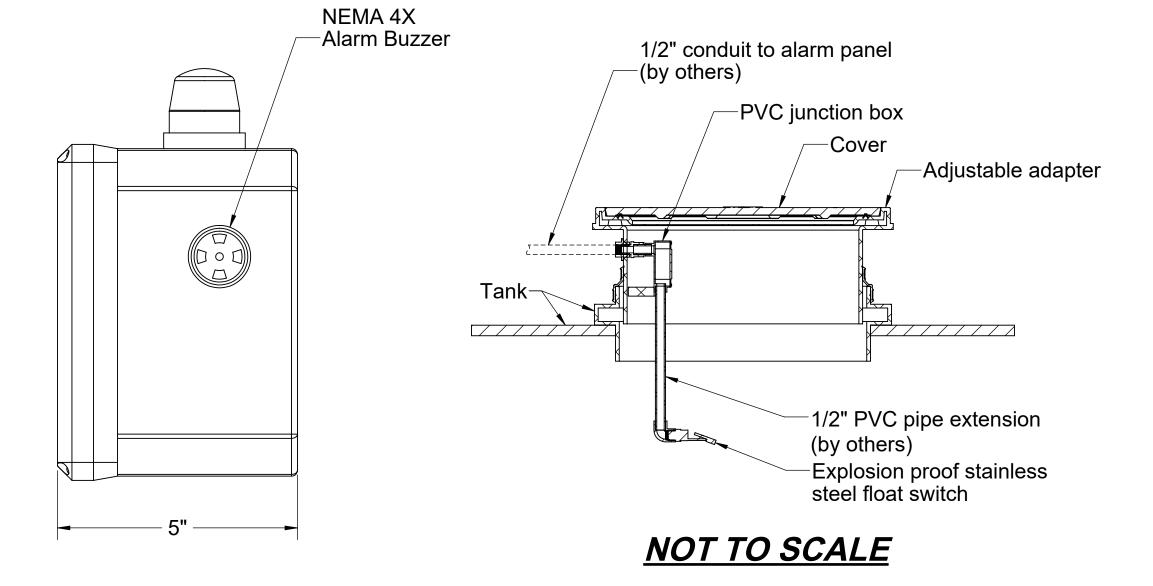
**DESCRIPTION:** HIGH LIQUID LEVEL ALARM WITH STAINLESS STEEL FLOAT SWITCH
