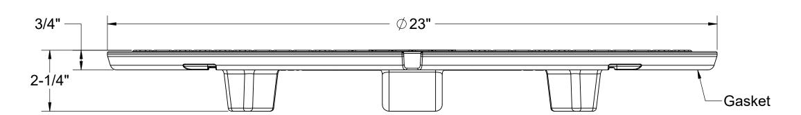
**SPECIFICATION SHEET DESCRIPTION:** 24" COVER PICKABLE CAST IRON H-20, HS-20 RATED
