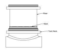
• Install risers and cover adapter into the tank neck starting from the marked riser, moving up to finished grade. Upper clamps may need to be loosened or
