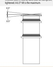
• If jobsite riser height conditions change after the previous steps have been completed, there is still room for vertical adjustment. • As long as the minimum engagement of 2-1/2" on all joints are maintained, the adapter and risers may be adjusted/cut as many times as necessary.
