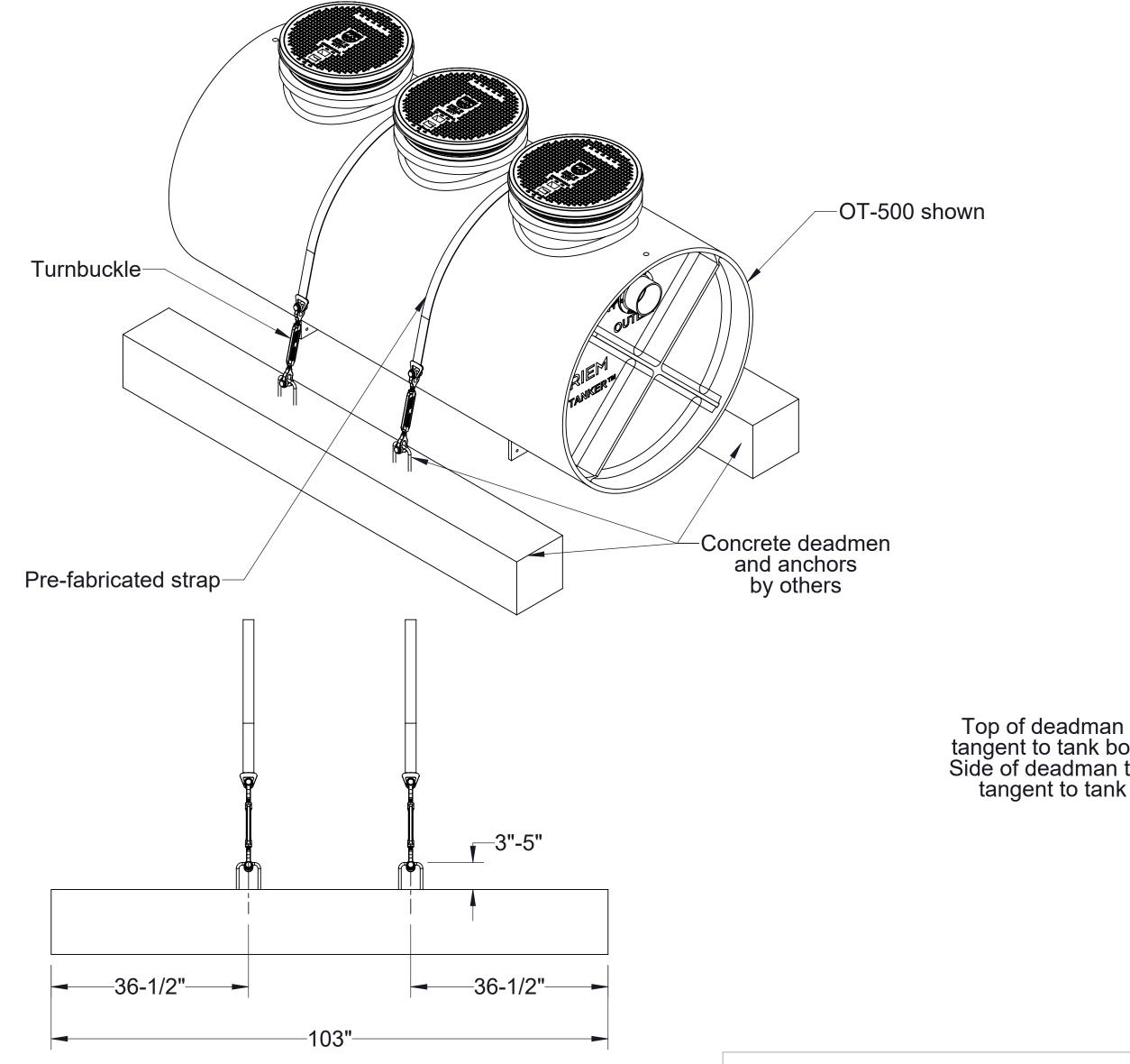
Top of deadman to be tangent to tank bottom. Side of deadman to be STRIEM tangent to tank side. OIL TANKER TWO -5-1/2" 49-3/4" 12"
