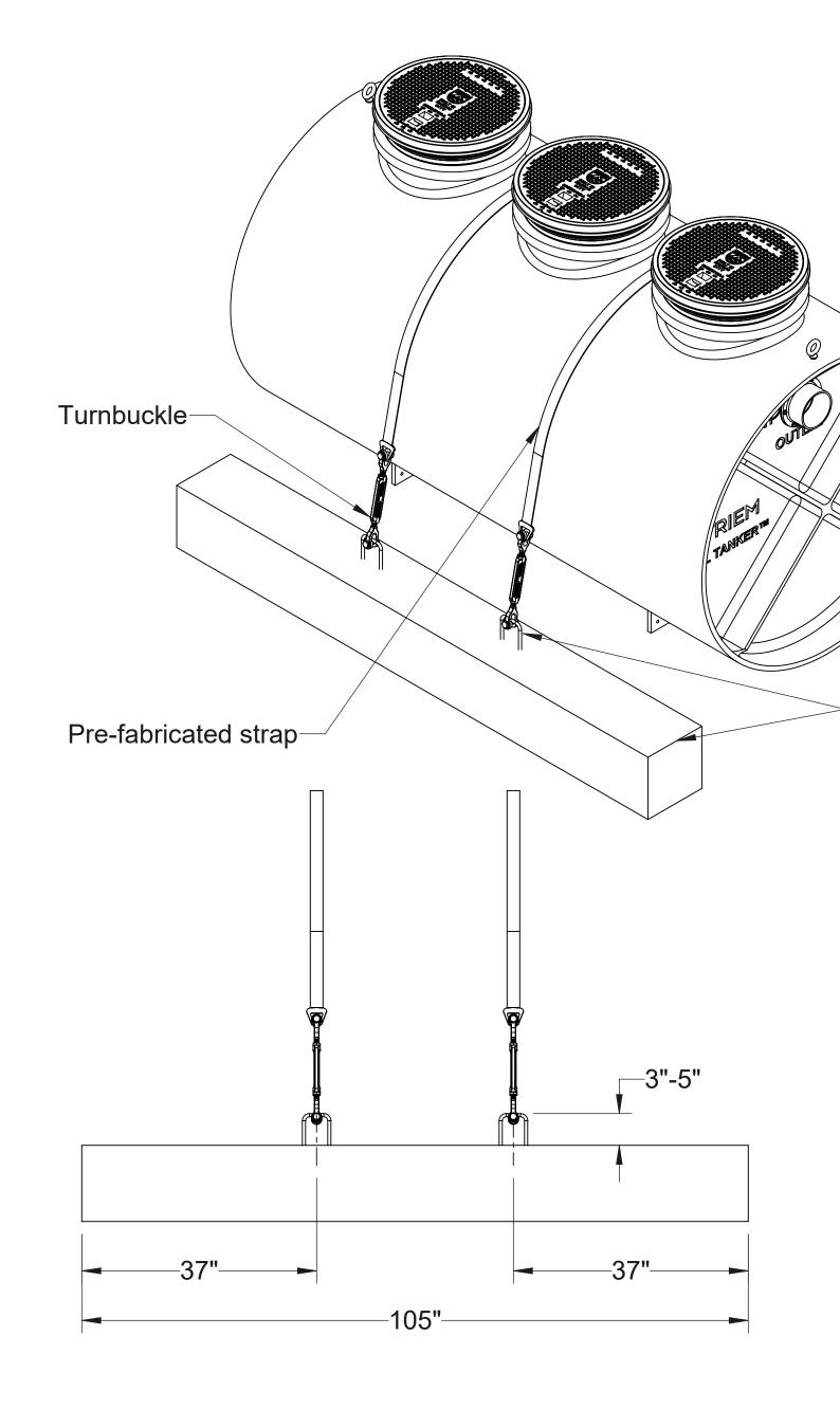
STRIEM Top of deadman to be tangent to tank bottom. Side of deadman to be tangent to tank side. OIL TANKER <del>---</del>5-1/2" 55-3/4"
