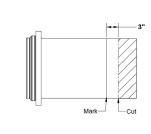
• Wipe clean all riser and cover adapter sidewalls. • Insert the first riser into the tank neck until the mark made in step 4 is in-line with the top of the neck gasket. This will ensure your risers reach the finished grade measured in step 1.
