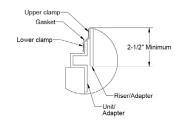
• Install risers and cover adapter into the tank
