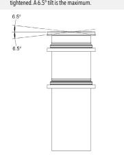
• If jobsite riser height conditions change after the previous steps have been completed, there is still room for vertical adjustment. • As long as the minimum engagement of 2-1/2" on all joints are maintained, the adapter and risers may be adjusted/cut as many times as necessary. Finished Grade
