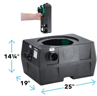
LB-15 OPTIONS 16" LS CC-1 CONNECTIONS: 2", 3" LIMESTONE LOAD: 200 LBS. # OF LAB SINKS: 4 COVER: PEDESTRIAN-RATED
