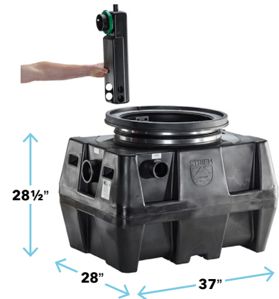
LB-50 OPTIONS TRAF 24" HDK LS CC-1 CONNECTIONS: 2", 3", 4" LIMESTONE LOAD: 650 LBS. # OF LAB SINKS: 15 COVER: PEDESTRIAN-RATED
