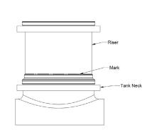
Install risers and cover adapter into the tank neck starting from the marked riser, moving up to finished grade. · Upper clamps may need to be loosened or removed to aid in assembly.
