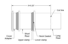
• Tighten all clamps to 14 lbs. of torque
