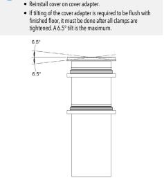
• If jobsite riser height conditions change after the previous steps have been completed, there is still room for vertical adjustment. • As long as the minimum engagement of 2-1/2" on all joints are maintained, the adapter and risers may be adjusted/cut as many times as necessary.
