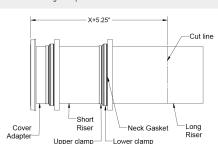
• Extend mark made in step 3 around the circumference of Cut along line with jigsaw, circular saw, or reciprocating saw. • Make a mark around the circumference of the riser 3" from the cut end of riser.
