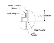
• Install risers and cover adapter into the tank
