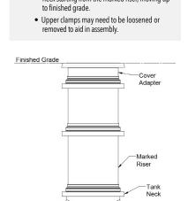
• Install risers and cover adapter into the tank
