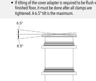
• Tighten all clamps to 14 lbs. of torque
