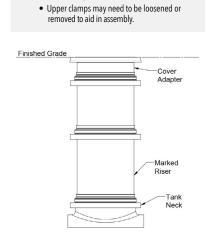
• Install risers and cover adapter into the tank
