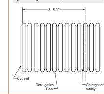
In the corrugation valley centerline that most closely precedes the mark from step 4, mark and cut along the centerline using the same method from step 3.
