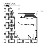
If corrugated pipe has an end piece, mark the corrugation valley closest to the end piece with china marker (included with tank).
