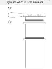
• If jobsite riser height conditions change after the previous steps have been completed, there is still room for vertical adjustment. As long as the minimum engagement of 2-1/2" on all joints are maintained, the adapters and risers may be adjusted/cut as many times as necessary.
