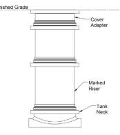
• Tighten all clamps to 14 lbs. of torque • Reinstall covers on cover adapters. • If tilting of the cover adapter is required to be flush with finished floor, it must be done after all clamps are
