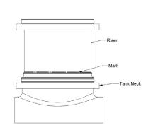
Install risers and cover adapters into the tank neck starting from the marked riser, moving up to finished grade. · Upper clamps may need to be loosened or removed to aid in assembly.
