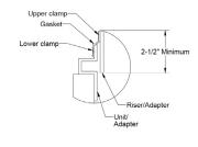
• Install risers and cover adapters into the tank
