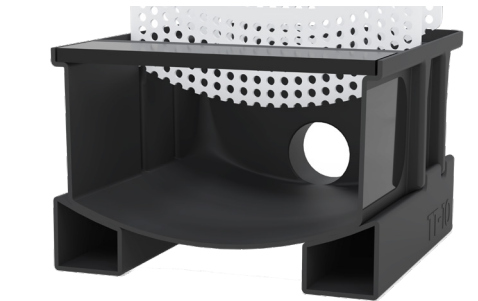
Internal floor is sloped toward outlet and is engineered with a parabolic shape to aid in flow evacuation and reduces solids buildup.
