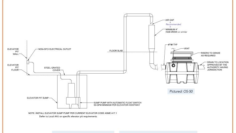
One Elevator, 50 GPM: OS-50 Two Elevators, 100 GPM: OS-100
