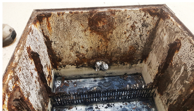
Pictured: Details of corroded steel tanks
