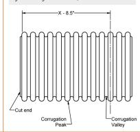
In the corrugation valley centerline that most closely precedes the mark from step 4, mark and cut along the centerline using the same method from step 3.
