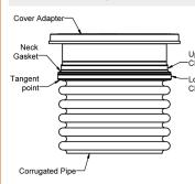
DO NOT AIR PRESSURE TEST UNIT! DOING SO MAY RESULT IN PROPERTY DAMAGE, SERIOUS BODILY INJURY, OR DEATH! Refer to Installation Instructions for correct testing procedure.
