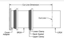
· Cut along line with jigsaw, circular saw, or reciprocating saw. . Make a mark around the circumference of the riser 3" from the cut end of riser.
